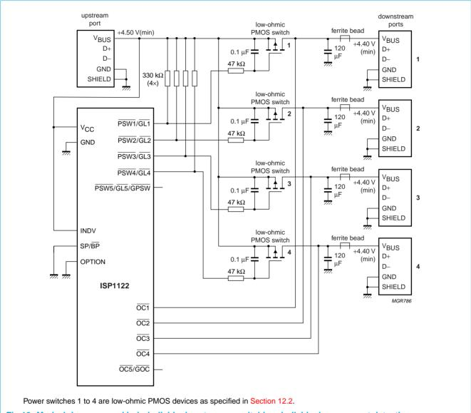
Fig 12. Mode 4: bus-powered hub; individual port power switching; individual overcurrent detection.
